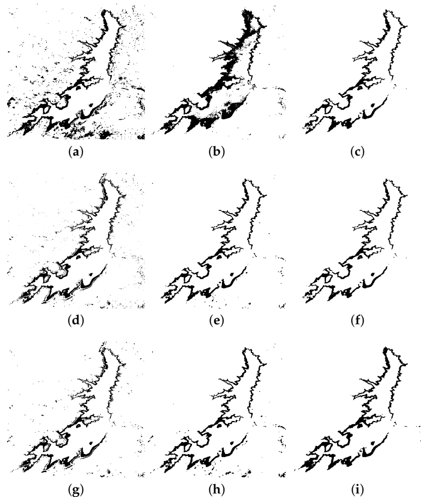
Figure 6. Change map of Itezhi Tezhi Dam, Zambia dataset (band 1) by (a) Normalized difference image (DI)+FCM (b) Ratio Image +FCM (c) Bandwise NSCT fusion +FCM (d) Bandwise NSCT fusion +SPSO (e) Bandwise NSCT fusion +PSOLF (f) Bandwise NSCT fusion +LIPSO (g) CVA (h) Transform change vector analysis (CVA)+LIPSO (i) Proposed NSCT feature fusion (All 4 bands) +LIPSO.
