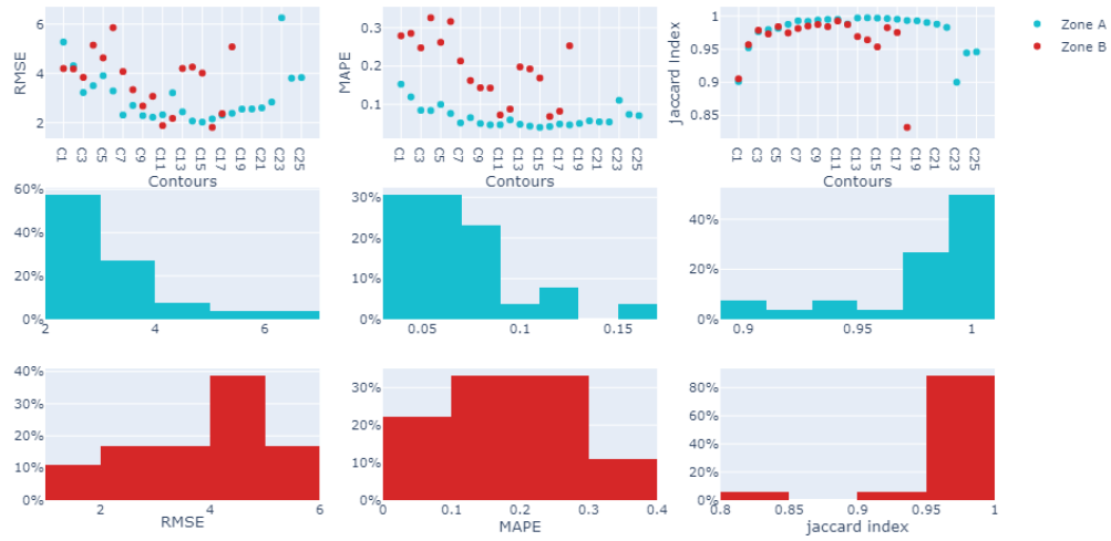
Figure 4-5: The figure depicts the RMSE, MAPE, and Jaccard Index value for each test contour for both case studies “Zone A” and “Zone B”; 2nd and 3rd row plots the percentage-wise distribution of interpolated test contours for RMSE, MAPE, and Jaccard Index values of “Zone A” and “Zone B” respectively, red color represents “Zone A” and blue represents “Zone B”.
